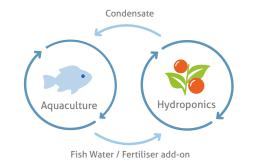
The double recirculation system provides optimized conditions for the fish and plant part independently from one another to increase the productivity of both.
